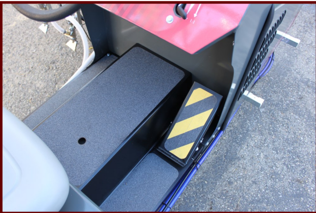
HYDROSTATIC DRIVE . SIMPLE HEEL AND TOW OPERATION
