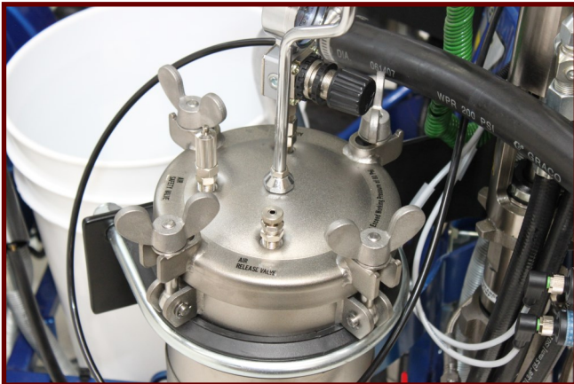
1/2 GAL SOLVENT AND CATALYST TANKS WITH GAUGES
