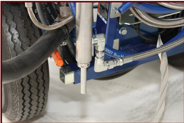
STAINLESS STEEL CATALYST PUMP WITH EXTERNAL INLET CHECK FOR EASE OF SERVICE
