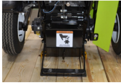
Large tilt up shroud for bit access
