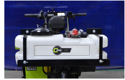
Dust suppression tank
